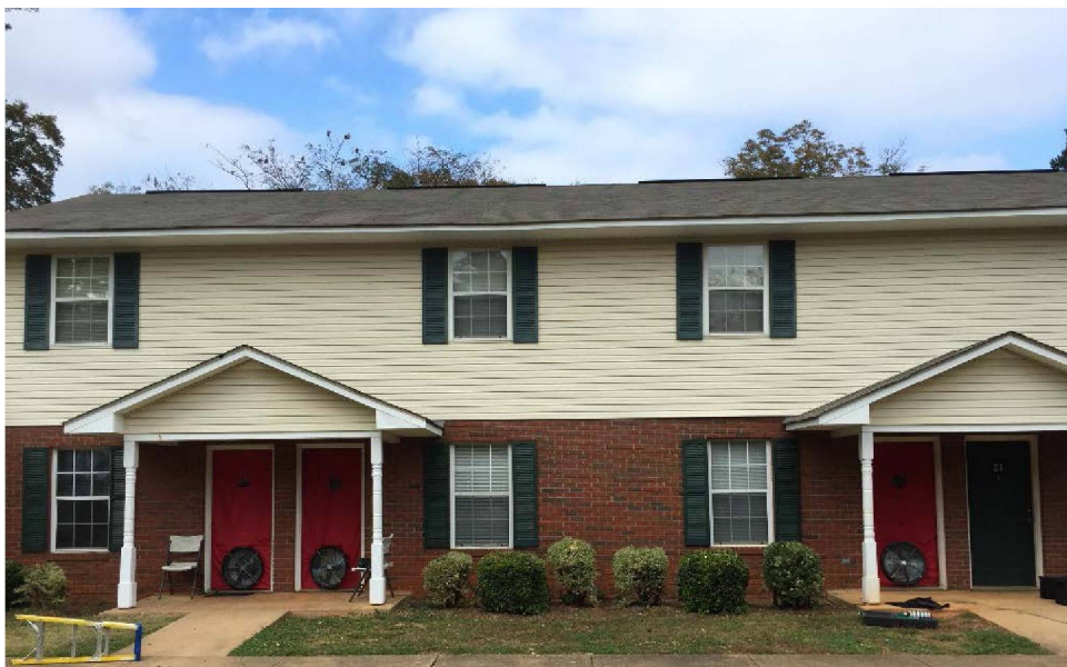
Figure 10. Configuration for guarded blower door test of center unit
