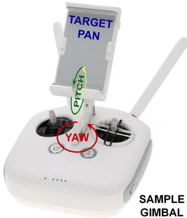
Figure 31. Illustration of a Two-gimbal Device Providing Yaw and Pitch Variability.
