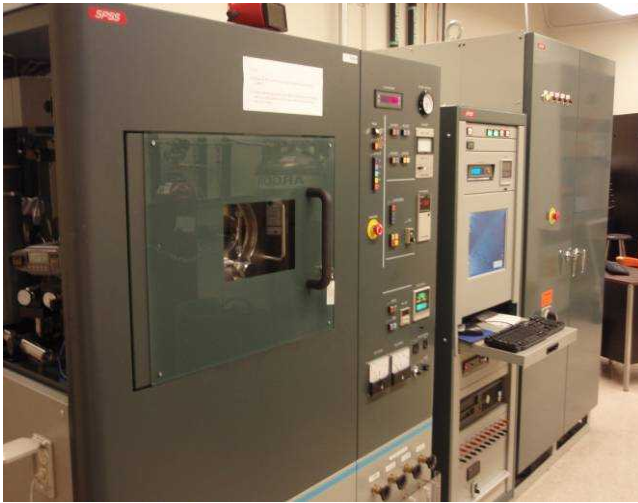
SPS Model: SPS-825S Dr. Sinter® at UCD
