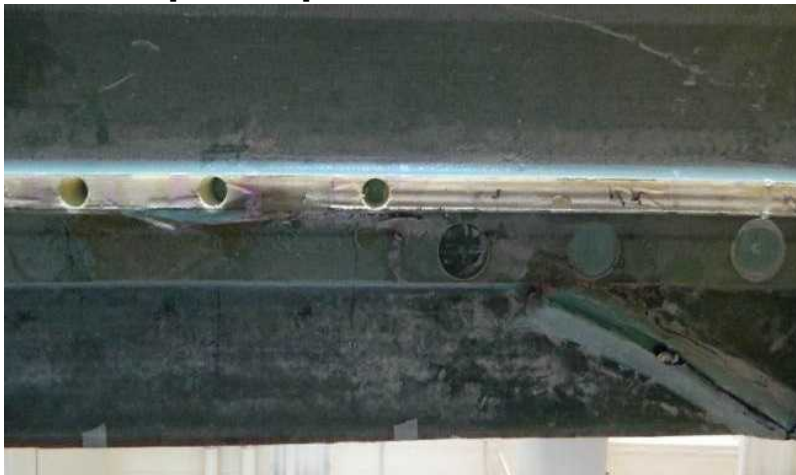
Spar Cap Cut From Blade
