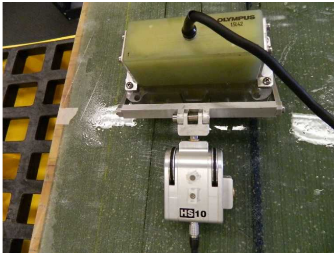
1.5L42 PA-UT Sealed Water Box with Mouse
