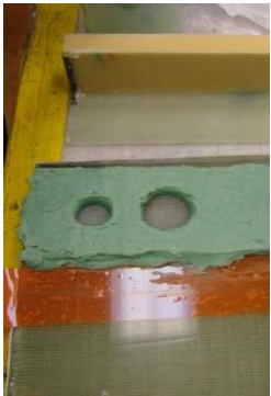
Voids in bond joint
