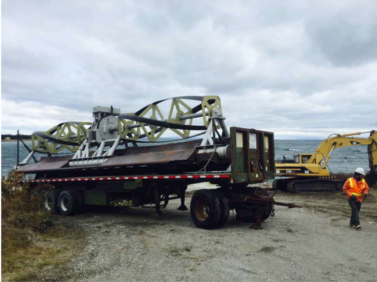
Figure 35: RivGen® TGU loaded on trailer in Igiugig and ready for transport to Homer on September 29, 2015
