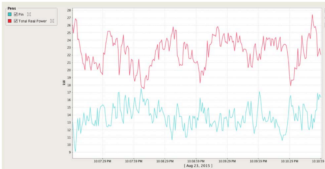
Figure 34: Output from the RivGen® Power System (blue) as compared to the Igiugig load supplied by the diesel generators (red) showing peak of 50% penetration around 10:08 pm on August 23, 2015
