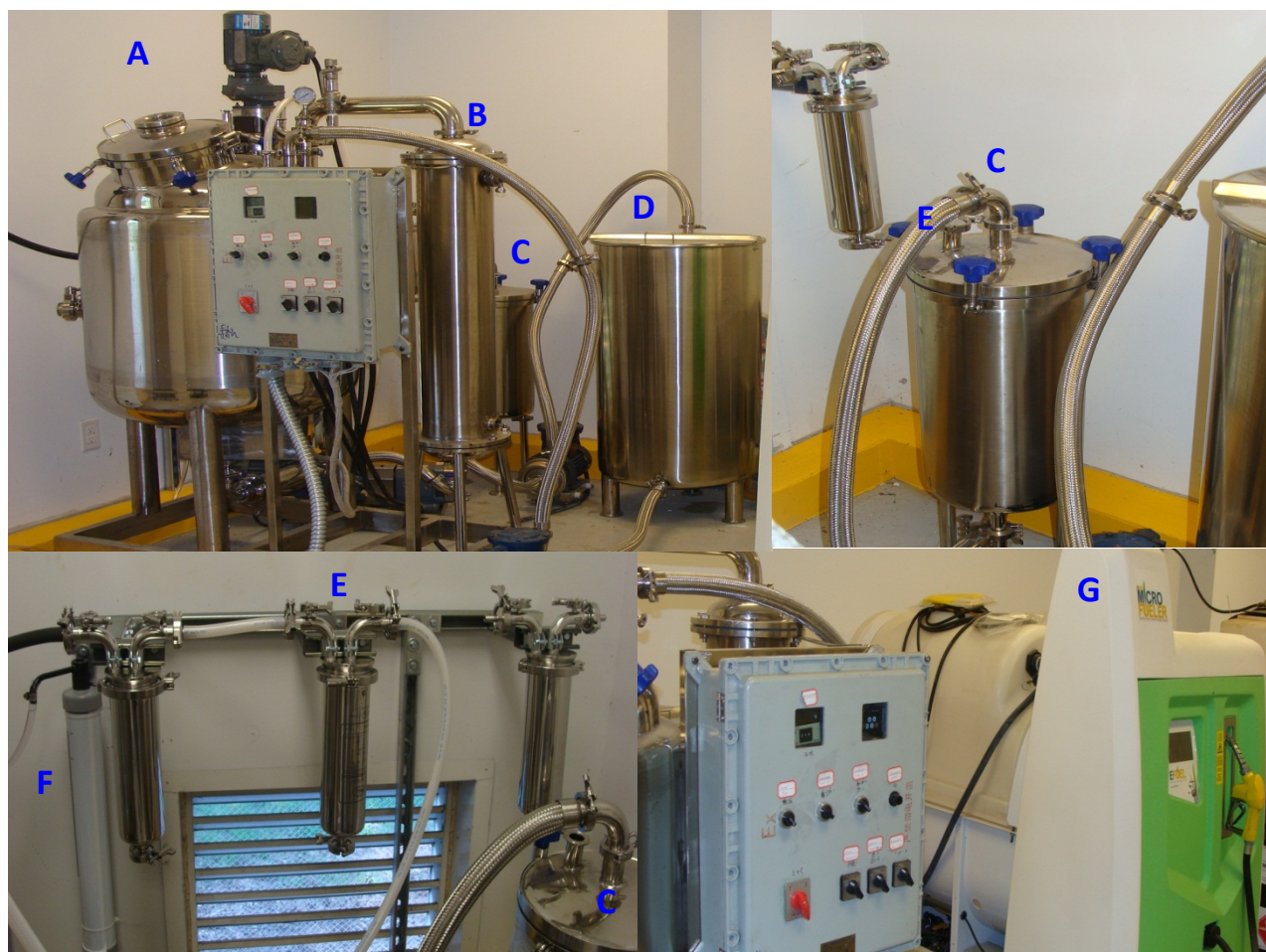
Figure 1: Highlights of installation of the farm deployable bioreactor system. Bioreactor (250 liters) for enzyme production, biomass treatment, saccharification, fermentation and ethanol recovery (A); Distillation condenser (B); Sand filter for separation of biomass and solids (C); Storage tank (D); Filter system for air purification (E); Water purification (F); and Microfueller for ethanol purification (G).
