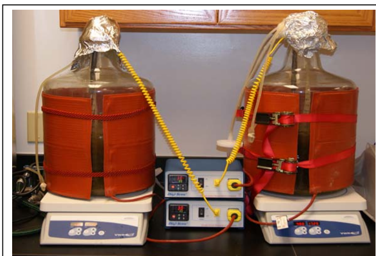
Figure 1. . Submerged fermentation for crude enzyme production in 20-L laboratory model bioreactor.
