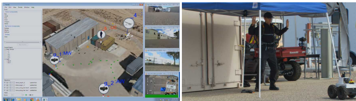
Figure 9. The GUI display when the intruder disappears under a blue tarp. The bottom-right live video feed shows that the intruder is no longer visible to the UAV (left). The intruder is then detected and confronted using a UGV (right).
