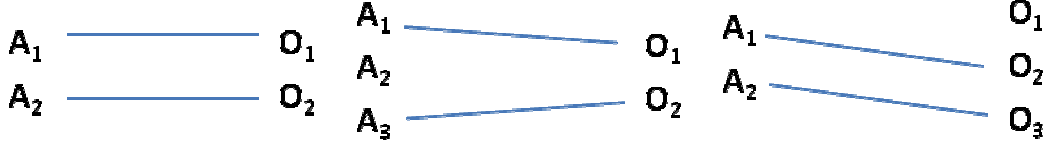
Figure 1. 1:1 assignment of agents to objectives when N_A = N_O , N_A > N_O , and N_A < N_O .
