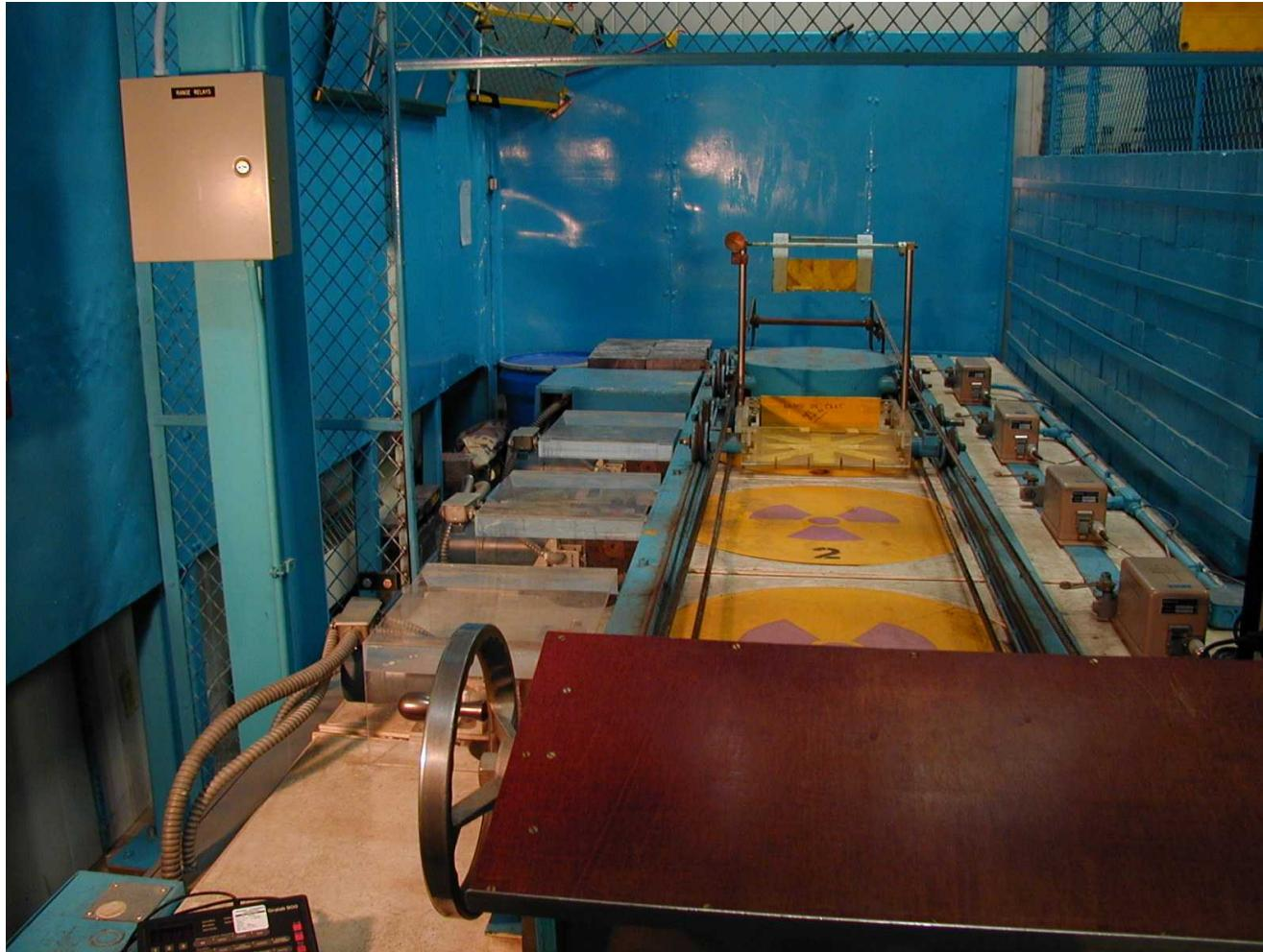
Four calibration source wells are used for calibration of exposure rate instruments from about 0.1 mR/h to 100 R/h
