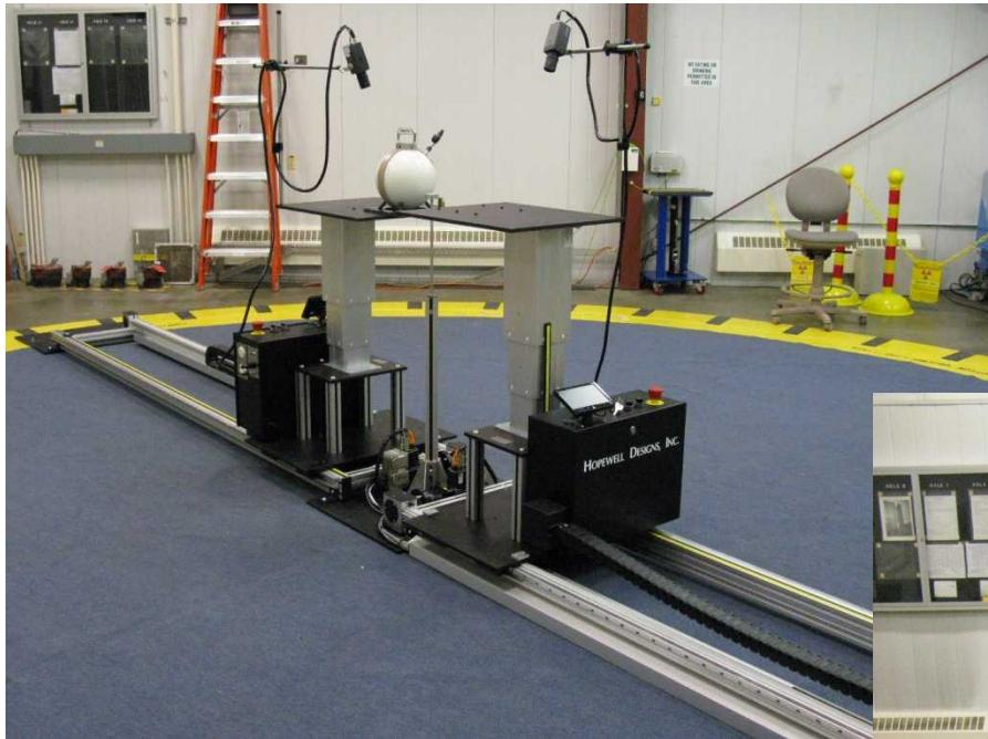
Neutron Source Range available for irradiation and instrument response evaluation. Laser-alignment is used to aid in device positioning. Cameras are positioned to remotely monitor instrument readings during irradiation.
