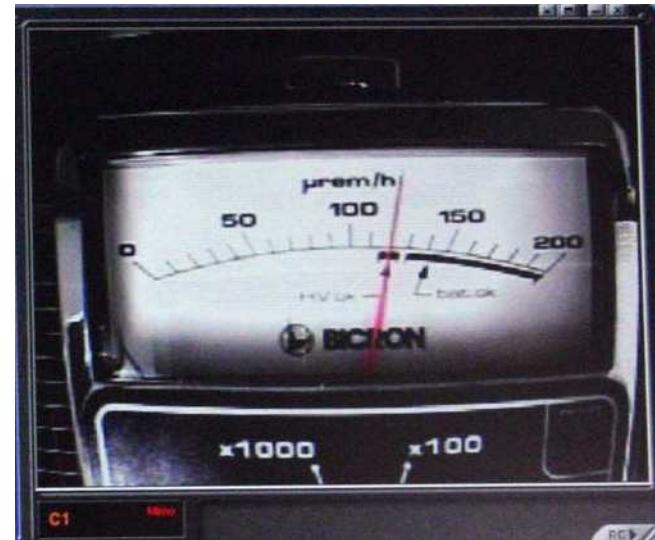
Monitor used to view the instrument as it is being calibrated.
