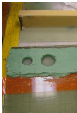
Voids in bond joint
