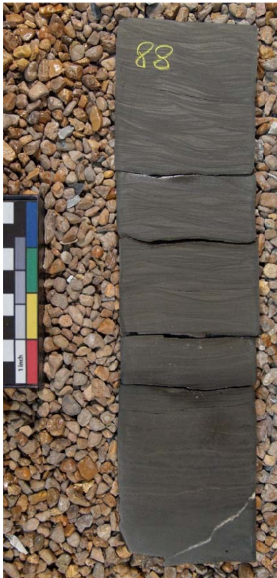
Depth 10688.5': A wispy laminated and cross-bedded siltstone.
