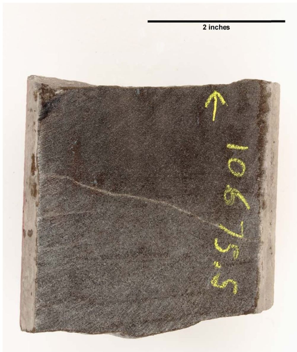
Depth 10675.6': A coarser, massive packstone. Open and cemented fractures are observed.
