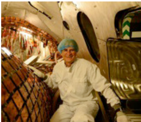
Glen Wurden in the stellarator's vacuum vessel during camera installation, with one hand on tile-backing plates and the other on a manned-entry port. Cameras capture images of the plasma effects on armored tile segments.
