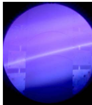
Using a high-resolution visible imaging diagnostic developed at Los Alamos National Laboratory, Glen Wurden took this single-frame, 30-ms-exposure image of W7-X's first plasma on Dec. 10, 2015. The image shows one of the five graphite limiters, visible behind the plasma as several tiled segments. He was one of six U.S. collaborators in the control room when the instrument came online.
