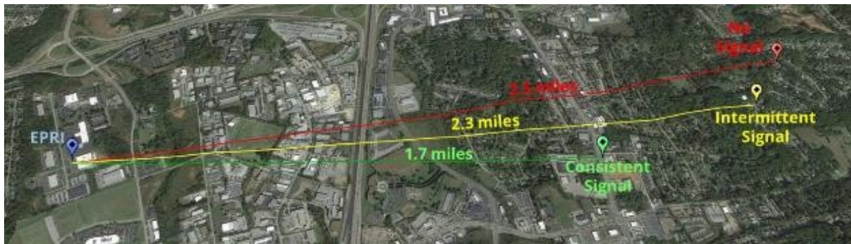
Figure 35 Summary of Field Tests with Remote Control Technologies 27MHz system
