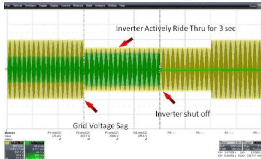
Figure 19 Inverter ride through and Shut-off test with 70% voltage sag
