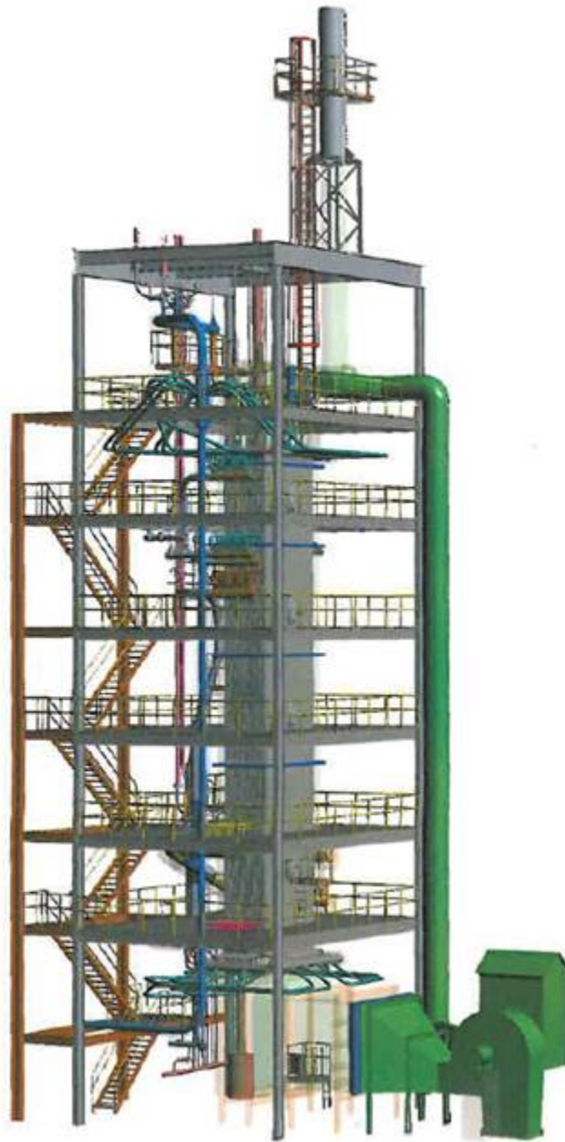
Figure 7-4 Babcock and Wilcox A-USC ComTest Superheater Tower 26 References
