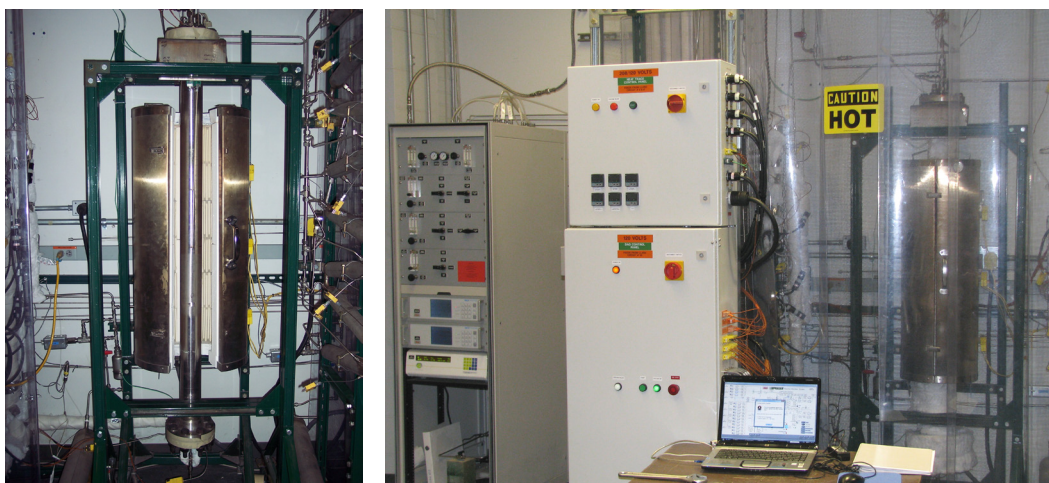
Figure 3, High-pressure reactor for testing OTM tubes at high temperatures, high pressures, and with sulfur containing impurities at Praxair, Tonawanda, NY.
