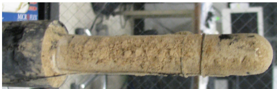
Figure 19: Accumulation of Ash Buildup on OTM Tube for Tests with Utah/PRB Coal Blend
