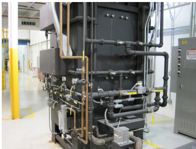
Figure 48: Pilot production furnace in Indianapolis illustrating H 2 /N 2 gas manifold.
