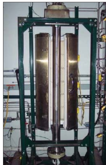
Praxair's high pressure reactor
