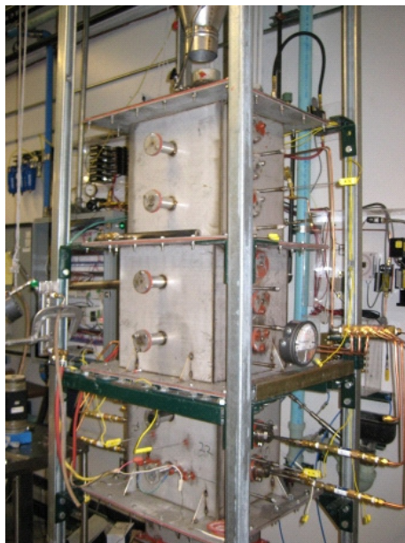
Figure 5, Multi-tube reactor for testing multiple OTM tubes in a coal environment at the University of Utah, Salt Lake City, UT.
