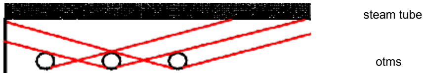
Figure 1: Radiation view factor geometry for elevation view, OTMs to steam tubes
