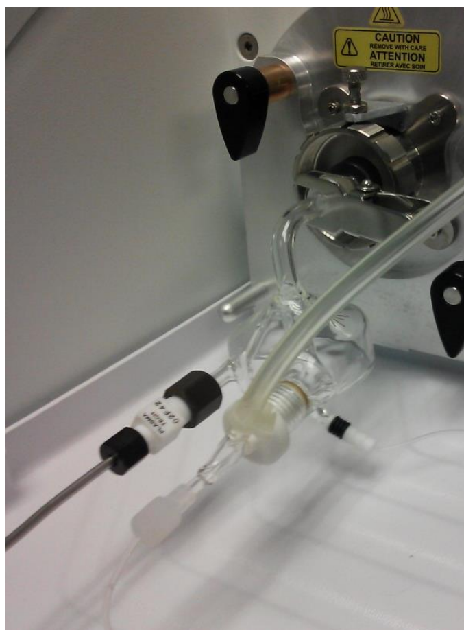
Figure 4: Dual inlet spray chamber. Inlet 1 (left) from He-jet with He flow rate of 1 L/min. Inlet 2 (right) from nebulizer that injects 200 \mu\text{L}/\text{min} of 1.00 ng/g In as an internal standard.
