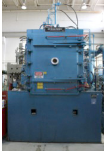
Left: MST-6 500-ton hydraulic press used to form components for the Lab's Hydrotest Program. Right: MST-6 heat treatment furnace used to heat treat components for the Lab's Hydrotest Program.
