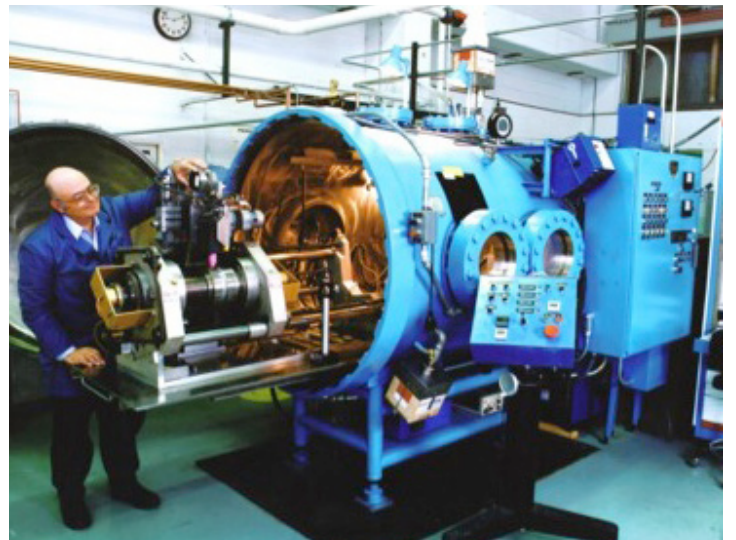
Semi-automatic gas metal arc welding equipment used by MST-6 to manufacture certain hydrotest components. Lab associate Paul Burgardt is shown in the photograph.
