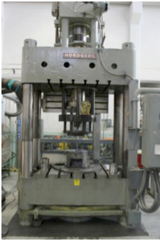
Left: MST-6 500-ton hydraulic press used to form components for the Lab's Hydrotest Program. Right: MST-6 heat treatment furnace used to heat treat components for the Lab's Hydrotest Program.
