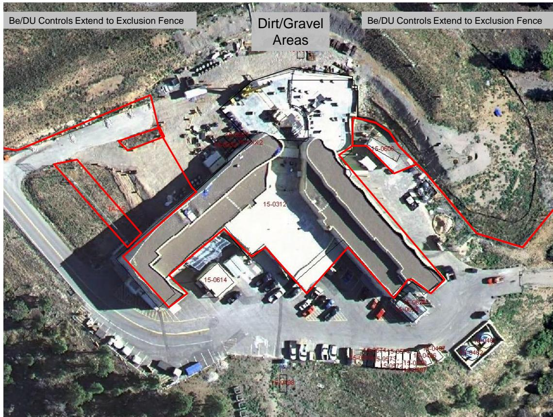
Figure 1: DARHT Be/DU potentially contaminated areas.
