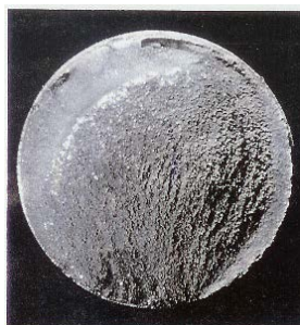
Bolt failure caused by hydrogen embrittlement.
