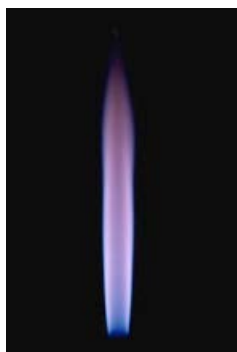
Hydrogen burns with a nearly invisible blue flame.
