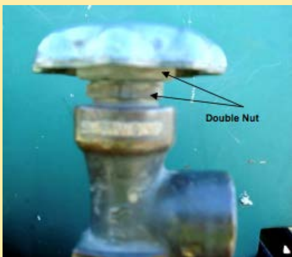
Figure 1. Leaking shutoff with a double-nut configuration.
