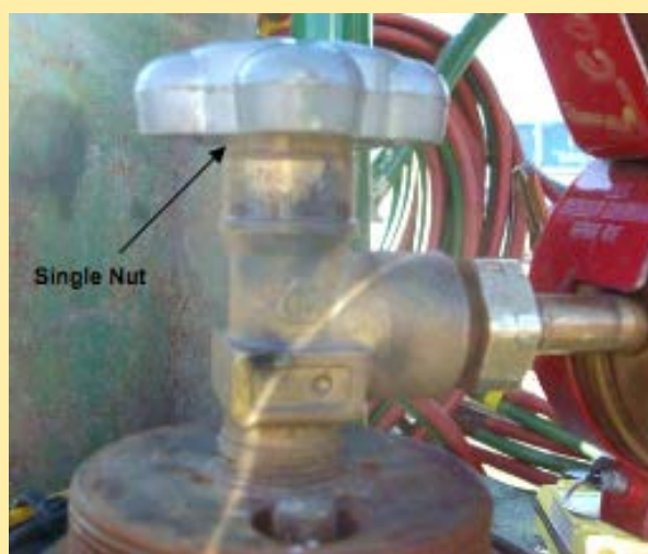
Figure 2. Nonleaking shutoff valve with a single-nut configuration.
