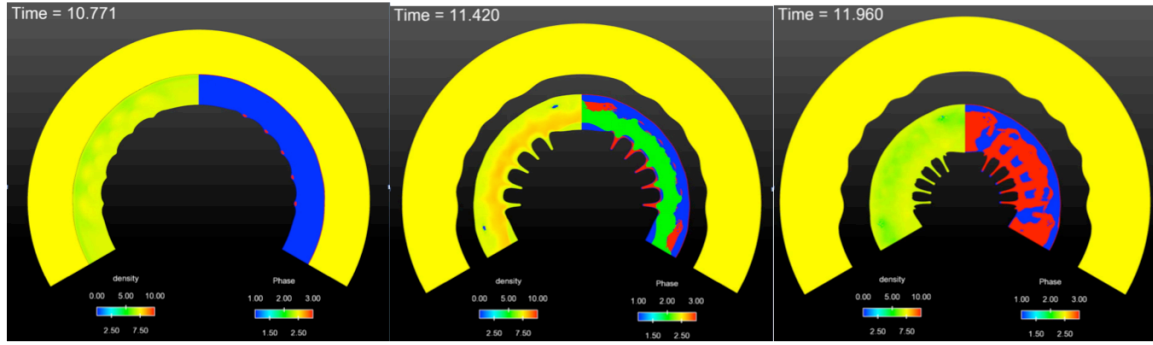
Figure 12. I = 0.8X , kA = 0.3 simulation. Spike release to liquid (red) but have their tips refreeze into the beta phase (blue) causing blunting at late time. The bulk transitions from beta to gamma (green) and liquid.
