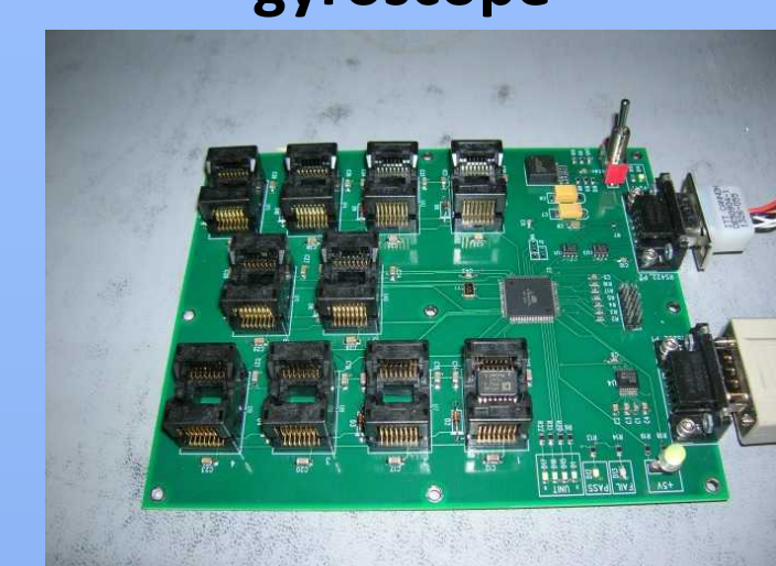
Test board- allows for simultaneous measurement of 10 chips
