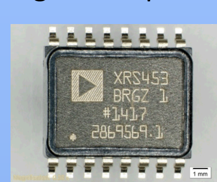
A Plastic Leaded Package (SOIC -package)
