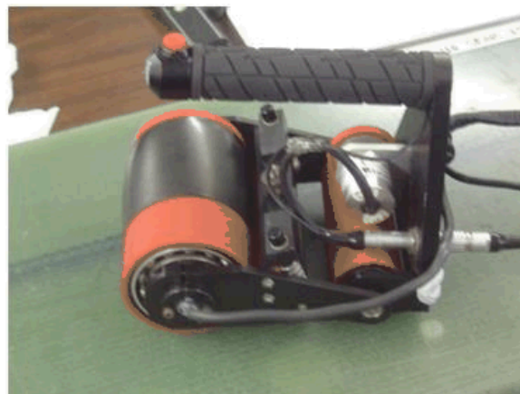
Figure 12. Sonatest RapidScan 2 – Linear Array UT WheelProbe Design.
