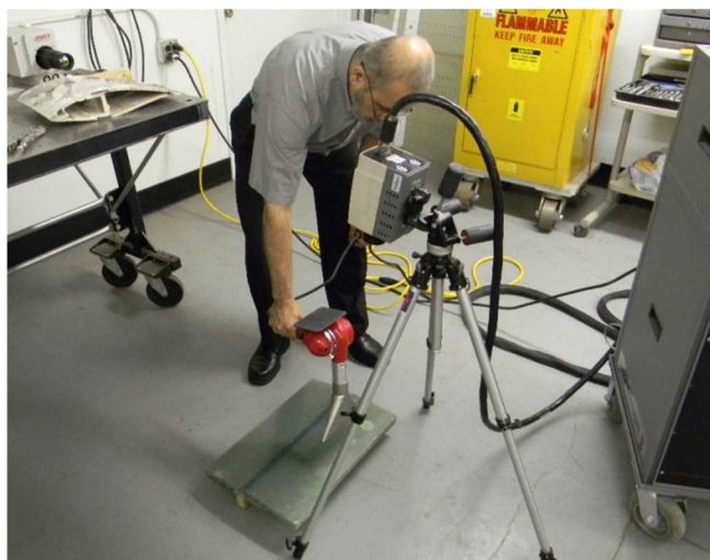
Figure 21. TWI Thermography System Inspecting a Wind Blade NDI Specimen.
