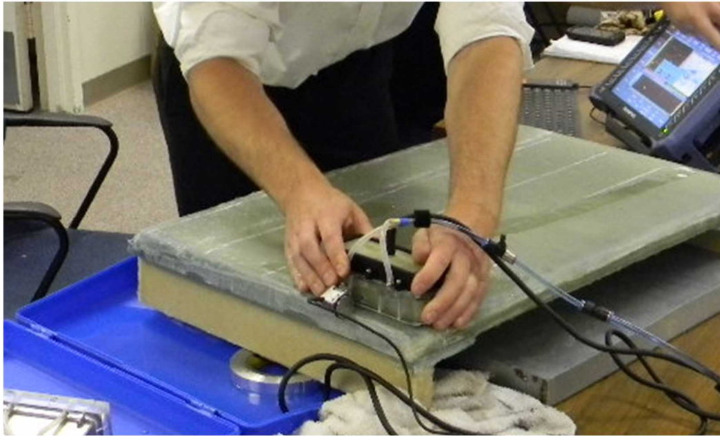
Figure 7. Phased Array Ultrasonics Inspection with OmniScan System.
