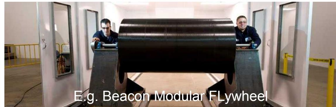
Carbon fiber materials / magnetic bearings
