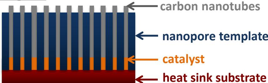
Starting material: Anodized aluminum oxide (AAO) nanopore templates on substrates
