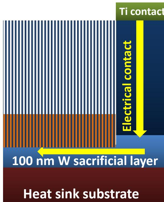
A sacrificial W “valve” layer oxidizes partially through during anodization. The  $\text{WO}_3$  is selectively removed to leave a conductive W layer at the pore bottoms. This facilitates catalyst electrodeposition, even on insulating substrates
