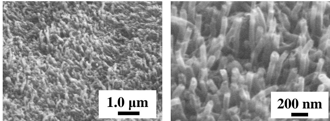
**Nanotubes are like cantilevers. Stress caused by vibration is largest near the pore mouth.**
