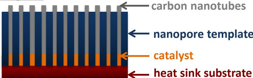
Catalyst for CNT growth: electrodeposited Co nanowires inside AAO pores
