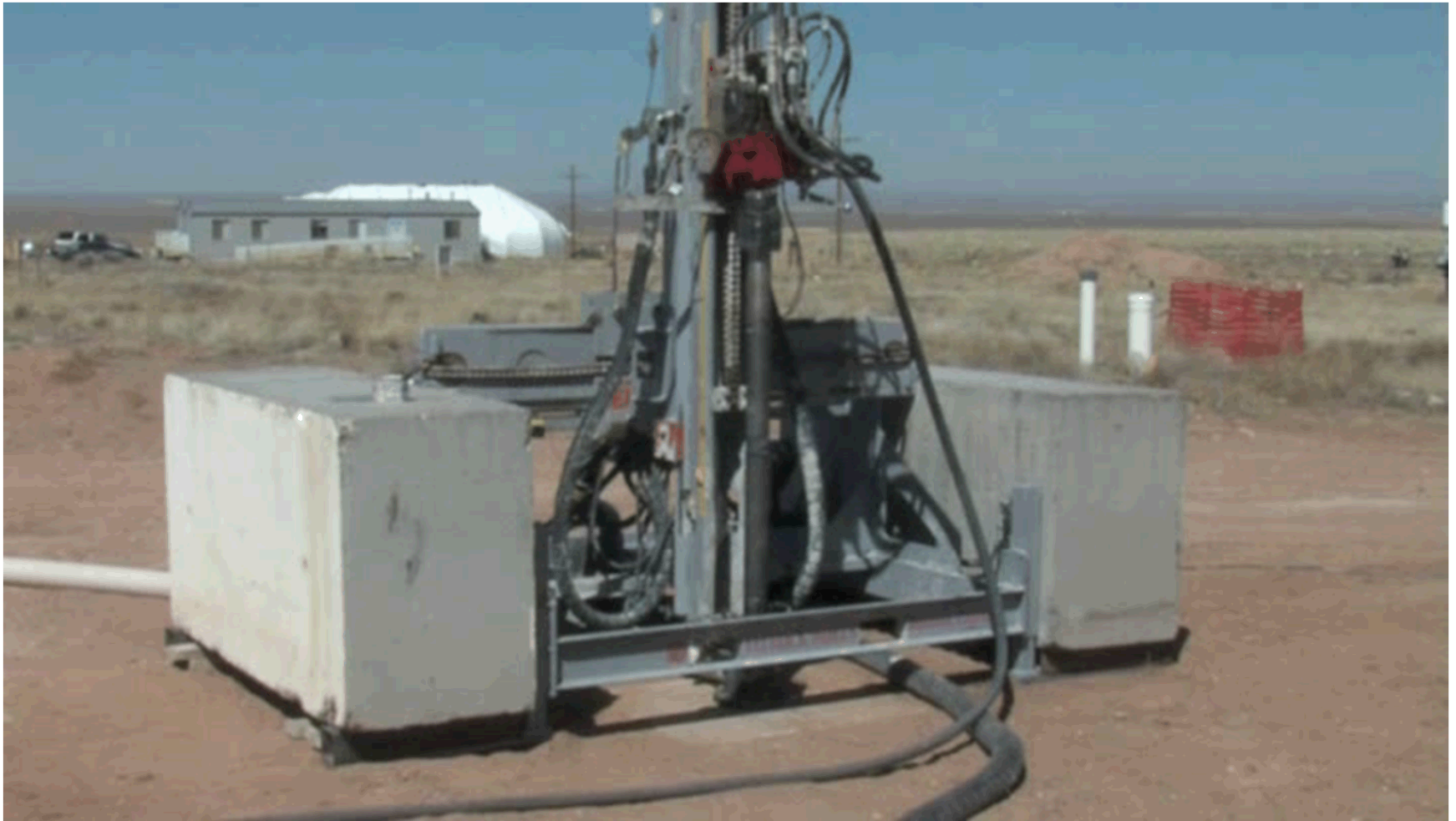
Drilling in 11-ksi, high-quality sandstone
