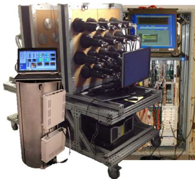
Figure 1: MINER (left) next to the larger neutron scatter camera and associated electronics rack. The digitizer and power distribution boxes can be seen on the side of MINER. Relative sizes approximate.
