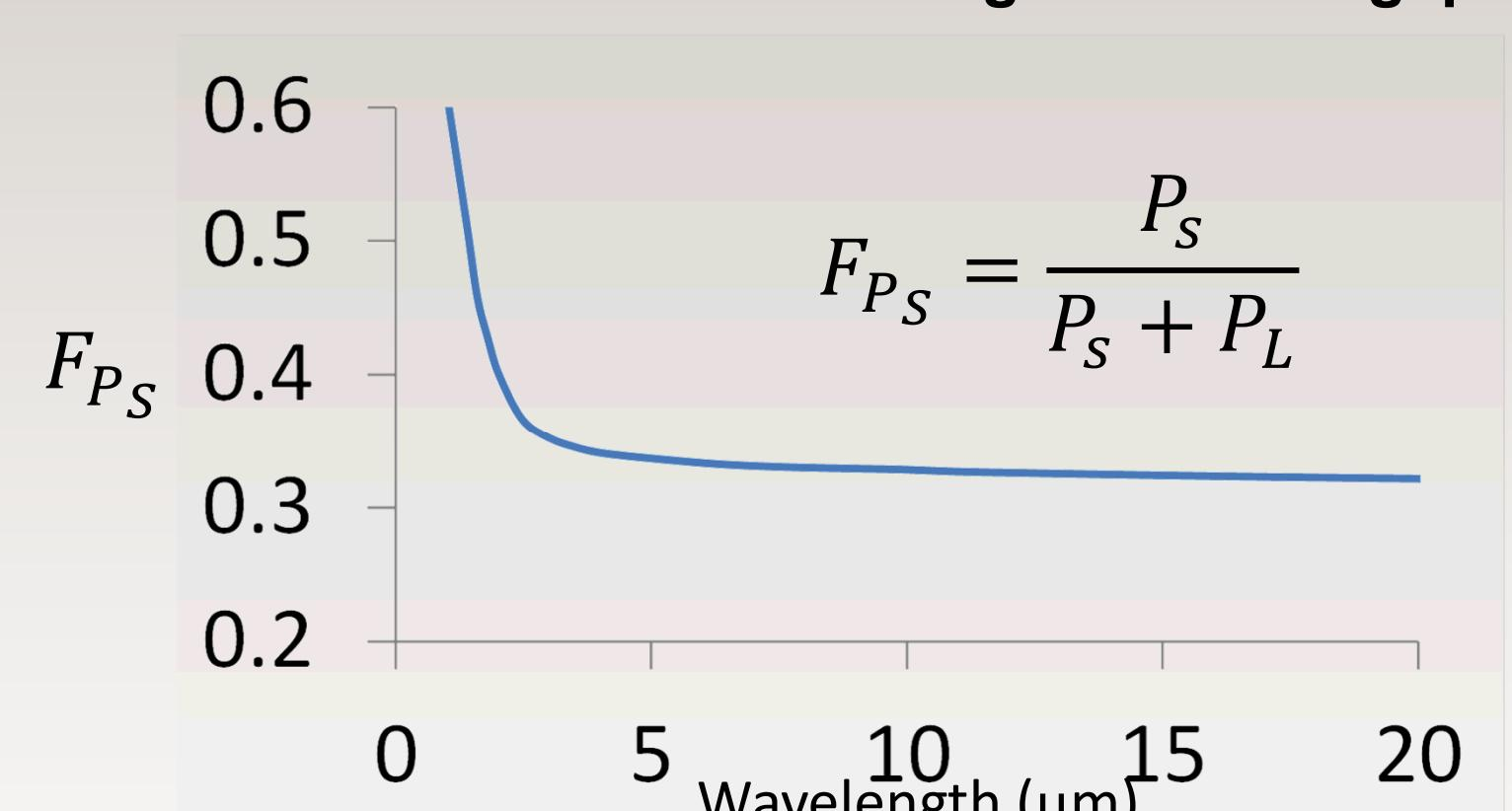
Surprisingly, nearly 30% of the transmitted power is channeled through an area  $\sim (\lambda/250)^2$  that is 1/60<sup>th</sup> of the unit cell area across broadband.
