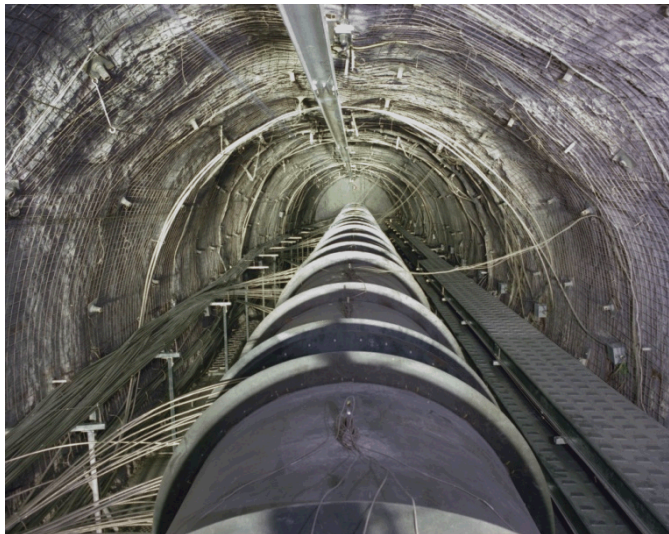
Drift Scale Test (9 simulated packages; ~200 kW)
