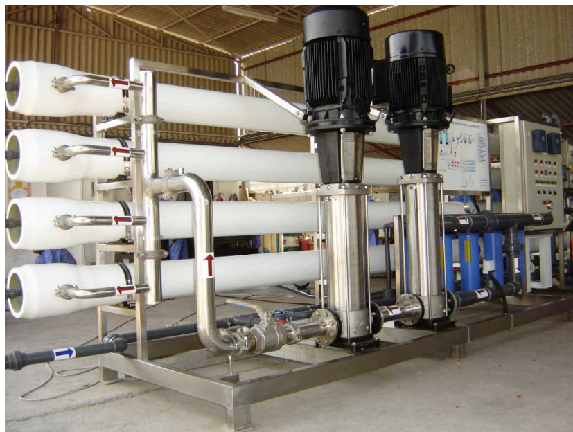
Figure 36. Reverse osmosis equipment at an industrial facility
