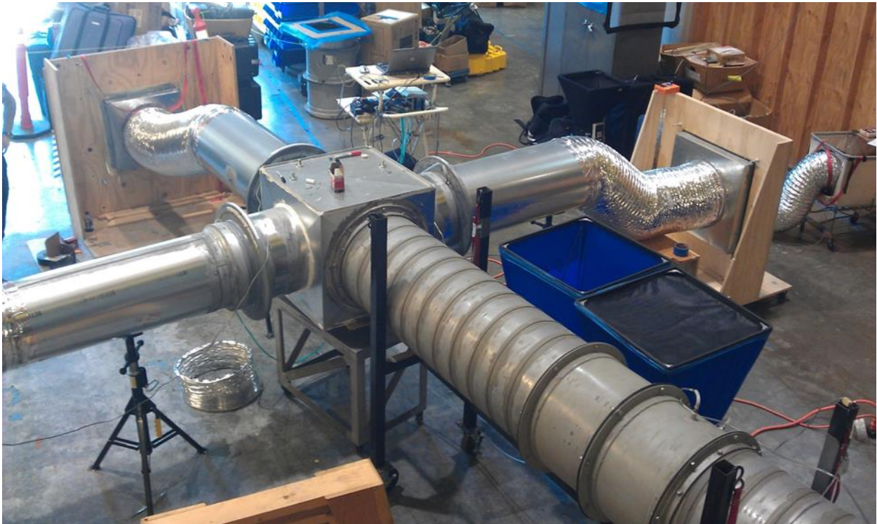
Figure 5: Multi-branch return flow experimental apparatus
