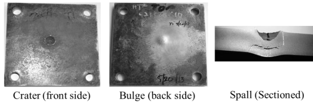
Figure 5: Typical target plate after impact (Test ID 1000-024)
