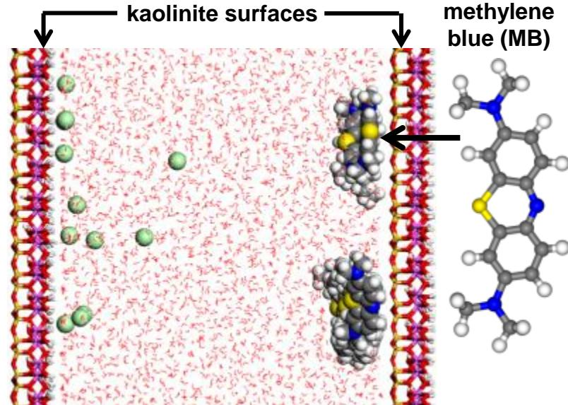
**MB adsorption in a kaolinite pore.** Partitioning of MB cations at the hydrophobic siloxane surface and chloride anions at the hydrophilic aluminol surface.
