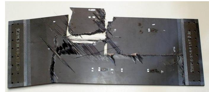
Typical crack growth in a notched laminate
