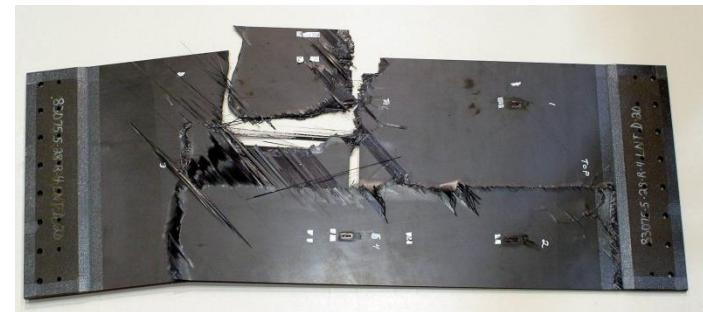
Typical crack growth in a notched laminate
