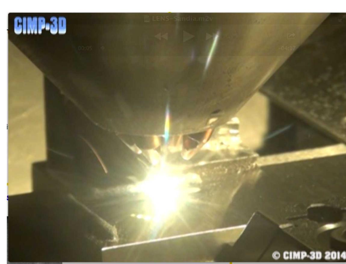
Photograph showing LENS® deposition of SS 304L
