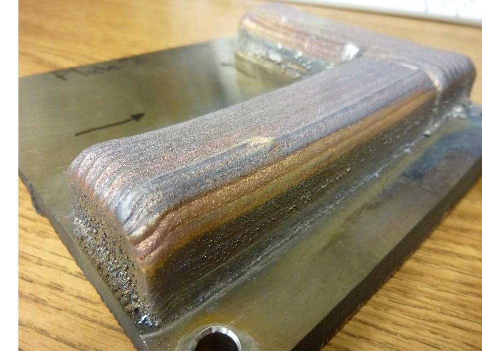
2.5 x 2.5 x 10 cm x and z bars by LENS® made from stainless steel 304L powder
