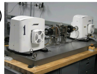
Used fuel rod stiffness Experiments (in hot cell and out) and analyses of stress distribution
