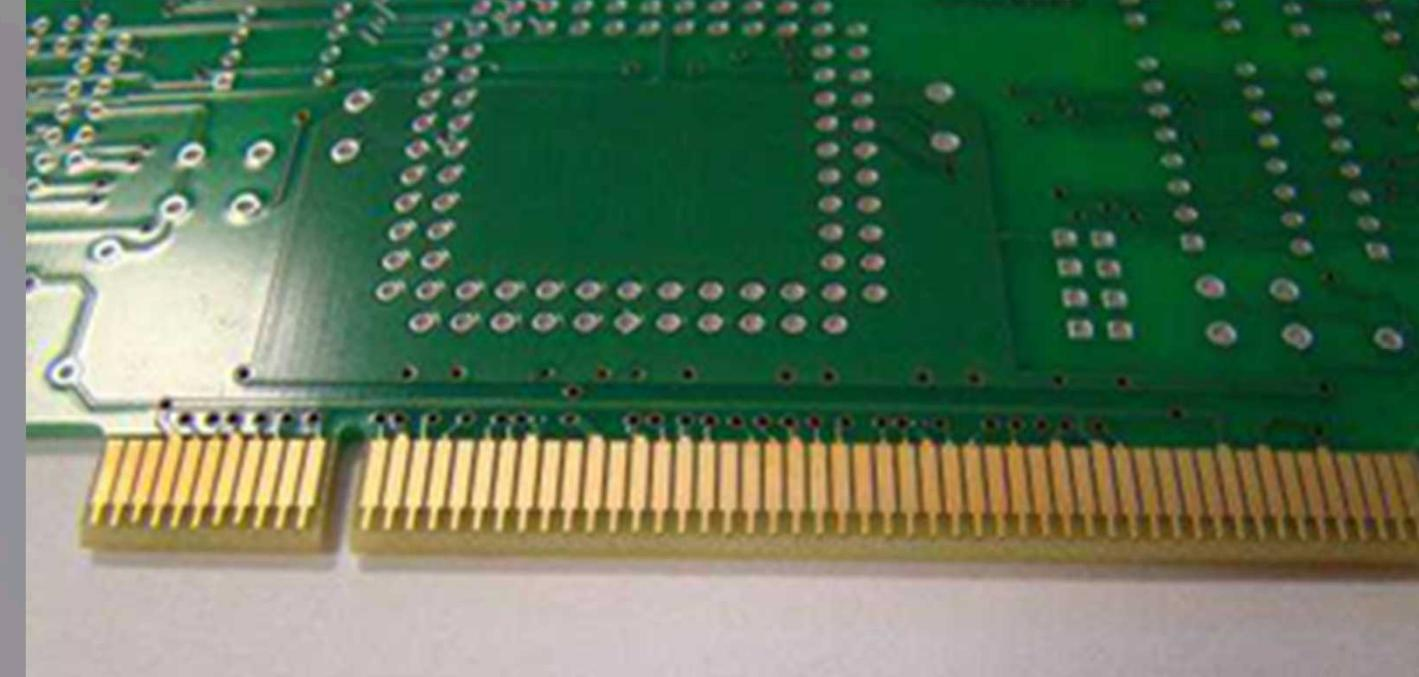
Gold has always been a preferred material in the electronics industry because it is inert and has very low resistance. However pure gold is too soft causing it to wear too easily and it has too high friction. This is why hard gold is used. Co, Ni, or Fe are added to the gold during electroplating, the dopants will fill the grain boundaries preventing grain growth. Because of the Hall-Petch relationship this will make the gold much harder and the resistance is still very low.
