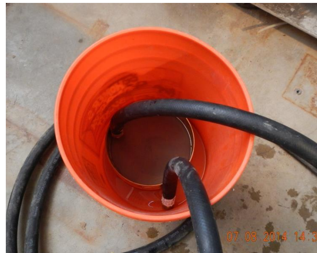
Flow that was drained was diverted through sieves for collection and weighing
