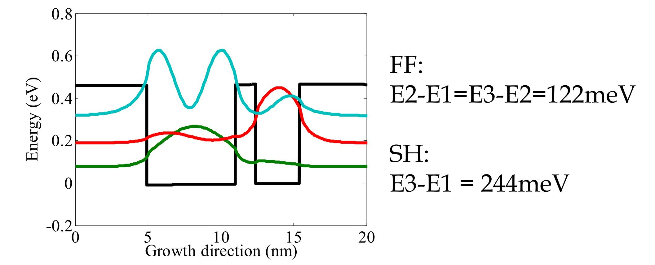
1-2, 2-3 transitions designed with equal energy (122 meV or 10  $\mu$ m) while maximizing oscillator strengths
