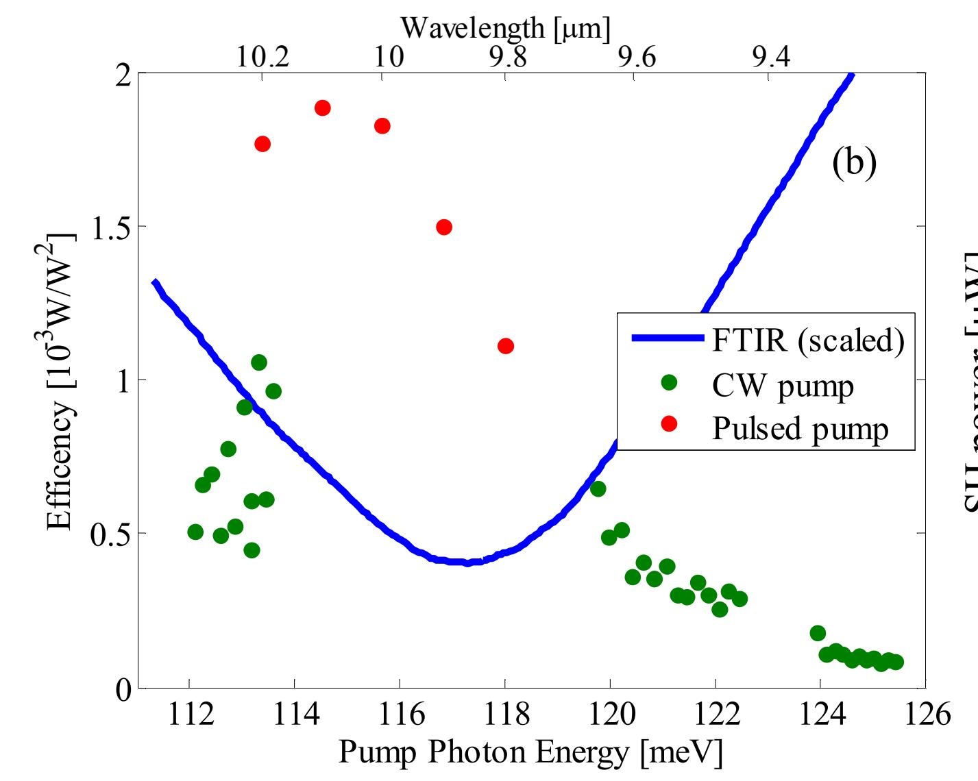
SHG efficiency shows strong frequency dependence as expected from resonant process and presented in ref[2]
