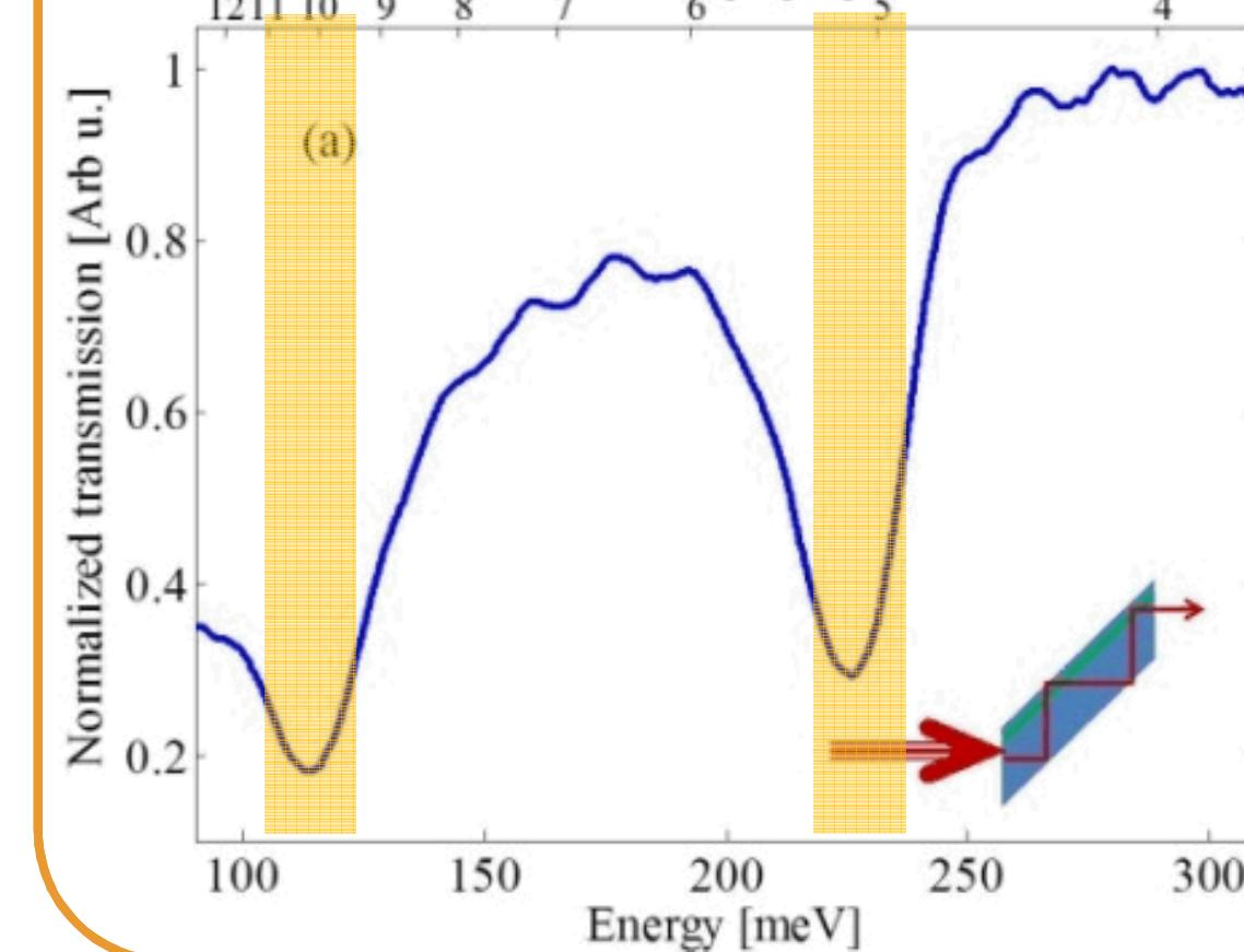
Absorption Dips correspond to 1-2 and 1-3 intersubband-transitions.
