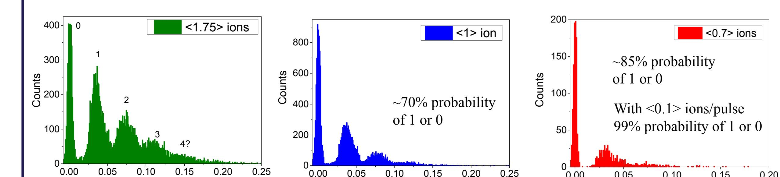
The quantization of ion number is clearly visible allowing for a determination of the CoolFET response per ion
