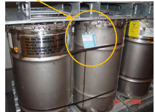
Deployed RF fiber optic seal security sensor on nuclear material containers
