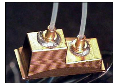
Although of lower per-unit cost, crimp-style connectors experienced an unusually high number of open circuits.
