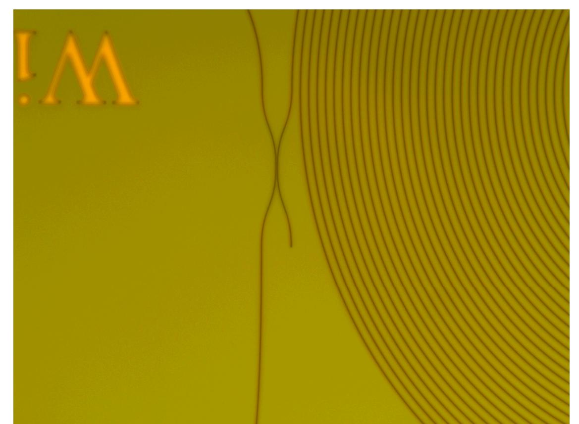
The integrated optics version of a beam splitter. Here it is used to construct a Mach-Zender interferometer.
