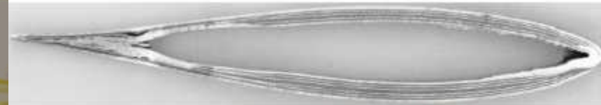
Figure 3 – Cross-section of the ORPC-supplied foil showing the laminate layup.
