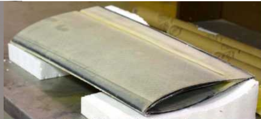
Figure 2 – Section of an ORPC-supplied foil, from which coupon substrates were cut.
