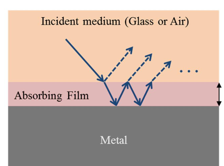
$$r = \frac{r_{01} + r_{12}e^{2i\theta}}{1 + r_{01}r_{12}e^{2i\theta}} \quad (\text{Airy's formula})$$
