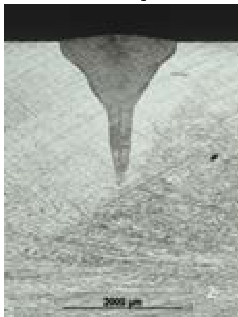
Figure 17: Expanded view of the +20 defocus weld in stainless steel generated at 20 mA with this LVEB machine.
