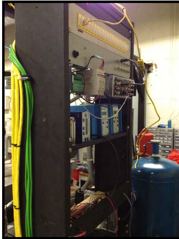
Figure 2-13: A picture of data acquisition system with temperature sensor wires, a modular data acquisition system, ETAS UEGO, Kistler 5010b, power relay, etc.
