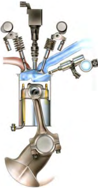
Figure 2-5: A diagram of the direct injection system on the LNF. Blue stream is intake air while red stream is exhaust. Image © General Motors.
