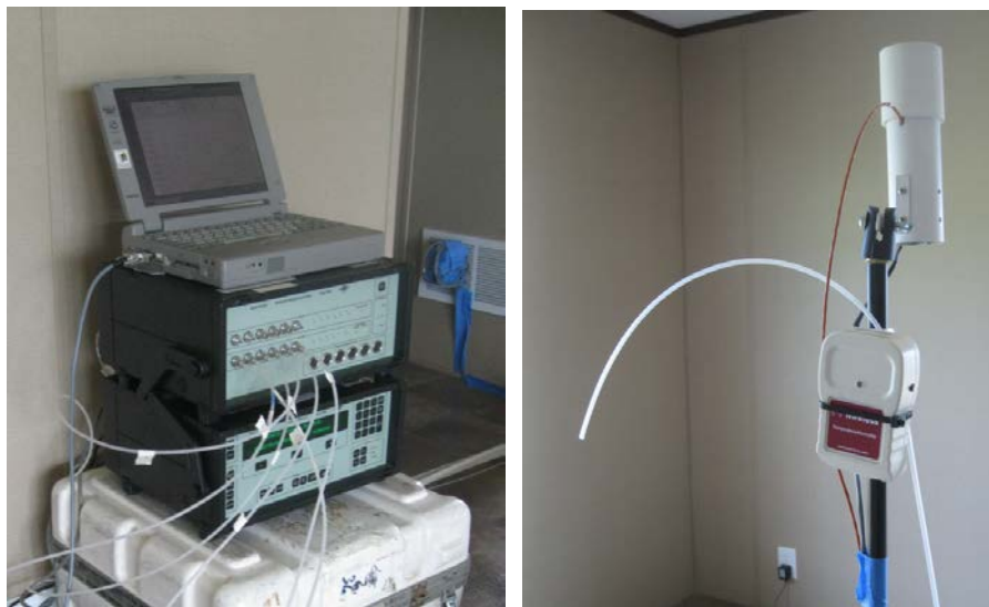
Figure 27. Tracer gas sampling equipment and sampling tube
