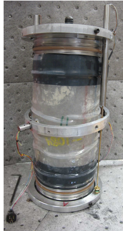
Fig. 1. Instrumented and jacketed specimen, this is axisymmetric compression specimen #11 post-test.
