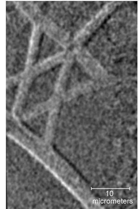
Nano-scale X-ray CT reconstructed slice through a few ligaments confirming the high quality of the print build.
