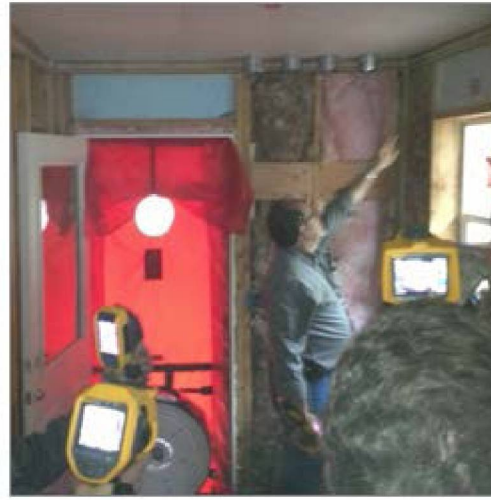
Fluke staff training HFH QA staff in the use of IR thermography to locate air leaks and insulation voids.
