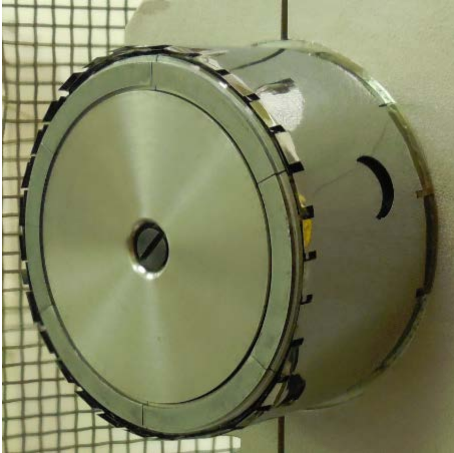
Figure 10. Photograph of electron gun emitter in a vacuum bell jar for initial testing
