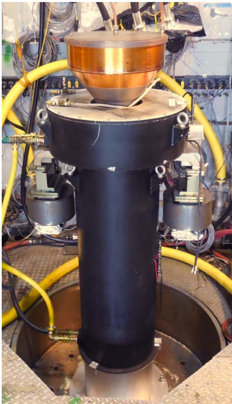
Figure 12. ABK mounted in the magnet, in the test set.
