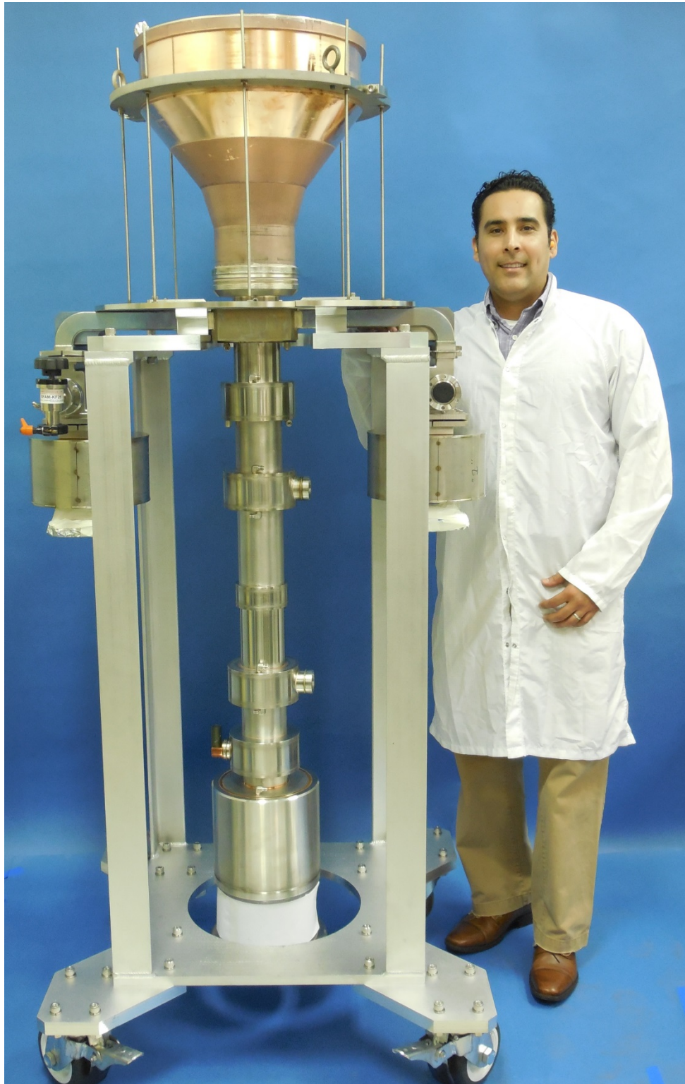
Figure 8. Annular beam klystron prior to bakeout.
